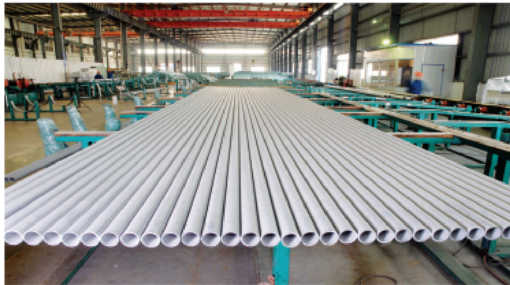
电站锅炉用不锈钢管 TP347H Grade TP347H of stainless steel pipe in the application of boiler of power station
