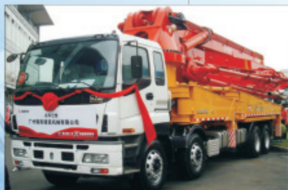
混凝土泵车 Concrete pump truck
