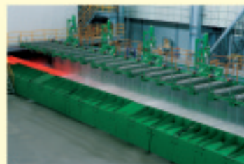
层流冷却 Laminar cooling
