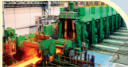
精轧机 Finishing mill
