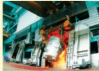
180吨顶底复吹转炉 180 ton top and bottom combined blown converter
