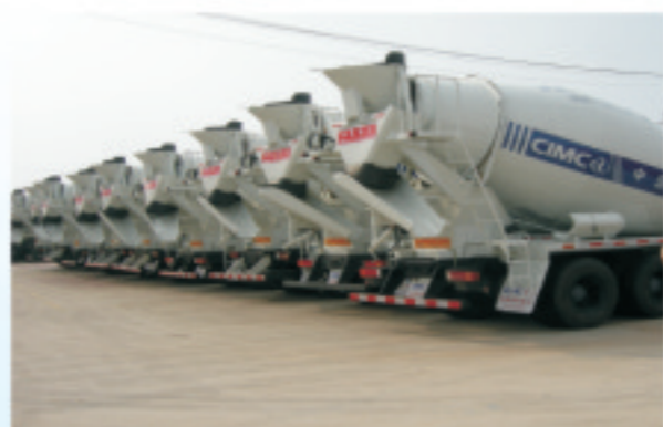
混凝土搅拌罐车 Concrete mixer truck
