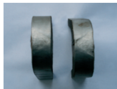
焊接接头弯曲试样 Welding Joint bending sample
